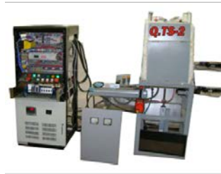
Thermal shock furnace at INCAS
