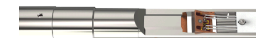
In situ double tilt heating holder containing MEMS heater chip (above) from DENsolutions (Delft, NL).
