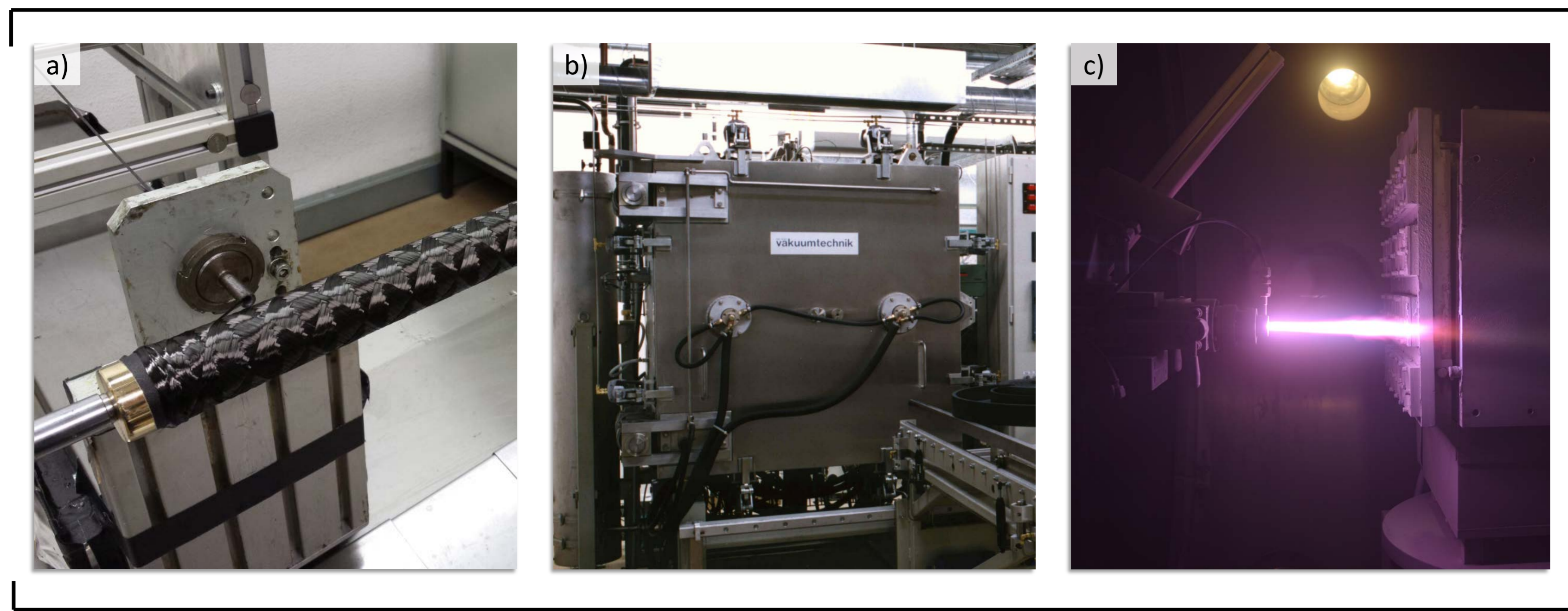
Fig. 1: Different techniques to manufacture nonoxide CMCs at DLR: a) filament winding process; b) furnace for pyrolysis and siliconisation; c) plasma spraying of environmental barrier coatings on CMCs
