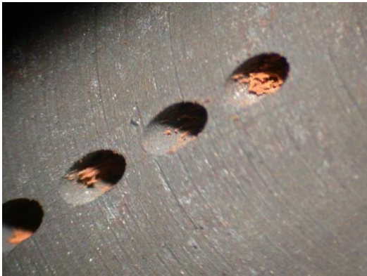
Fig. 6.6 – Deposition in first four cooling holes of HD45, 1050°C
