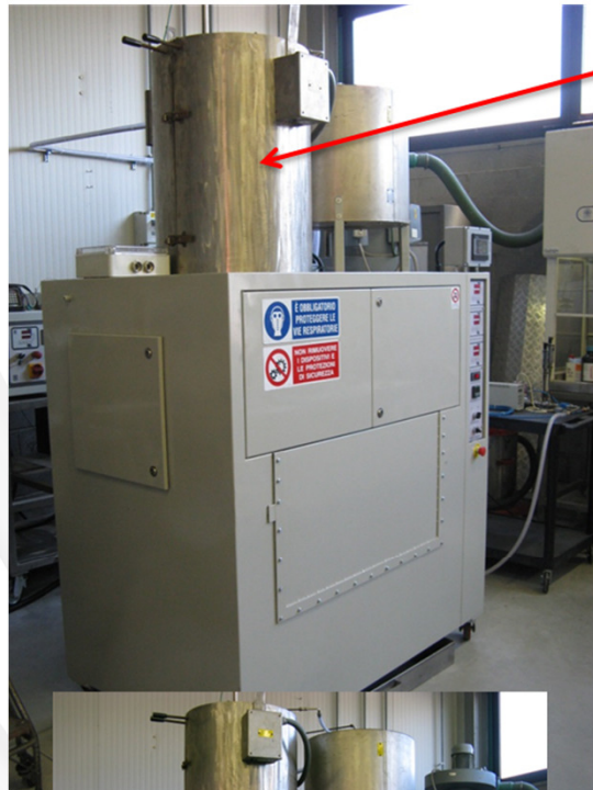
Main furnace with the coil for air inside
